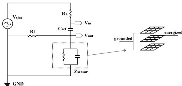
Figure 2. Simplified schematic of the sensor circuit and parallel plates (adopted from Yang et al., 2013a).
